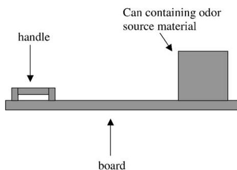
Fig. 1. Diagram of apparatus used to present odors to dogs.
